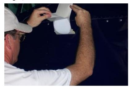
6. Using a squeegee or credit card, slowly work from the tape hinge side and rub the decal onto the surface. A side-to-side motion and moderate pressure will help reduce air bubbles under the decal.
