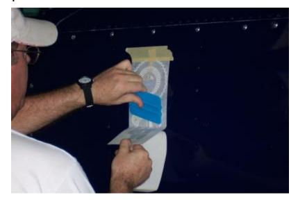
8. Slowly peel the top application tape away from the decal at a low angle (close to the surface). Avoid pulling straight up and lifting the decal or inducing bubbles. If any areas of the decal try to lift, stop pulling the application tape and rub the area back down with the squeegee and try again.
